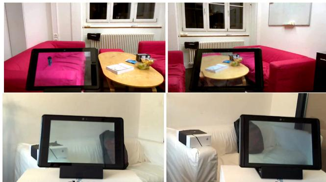
Fig. 7. Examples of view correction results from our system, as seen by the observer. Top: Fixed relative observer pose. In the left image, an AR object is rendered into the view. Bottom: Dynamic observer pose with two tablets (*c.f.* Sec. 4.2.2). We show these experiments in action in the supplementary video.
